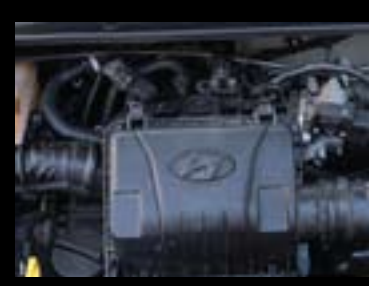
Eon's 814cc engine is basically the Santro engine, but minus one cylinder. It's only an average performer
